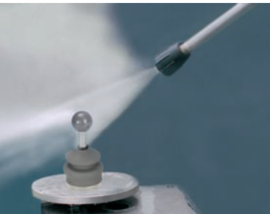
Protection class test IP 69K: in addition to the test for dust proofness, the test for IP 69K (originally intended as the protection class test for road vehicle construction) specially simulates the resistance to high-pressure cleaning of devices by splashing the tested devices at approx. 5 revolutions per minute under high pressure (approx. 100 bar) with an 80 °C -hot jet of water without causing any damage.
