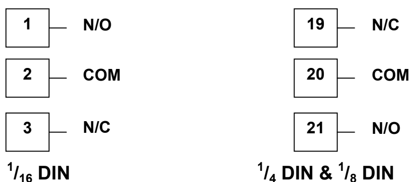
Figure 18. Option Slot 1 – Relay Module
