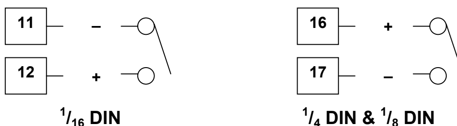
Figure 33. Option Slot A – Digital Input Module
