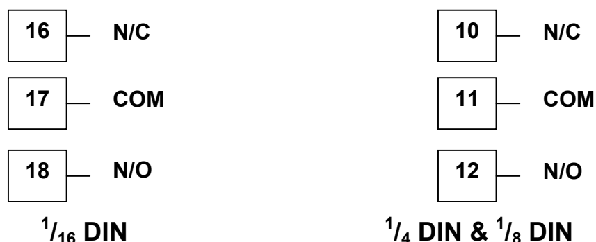
Figure 27. Option Slot 3 - Relay Module
