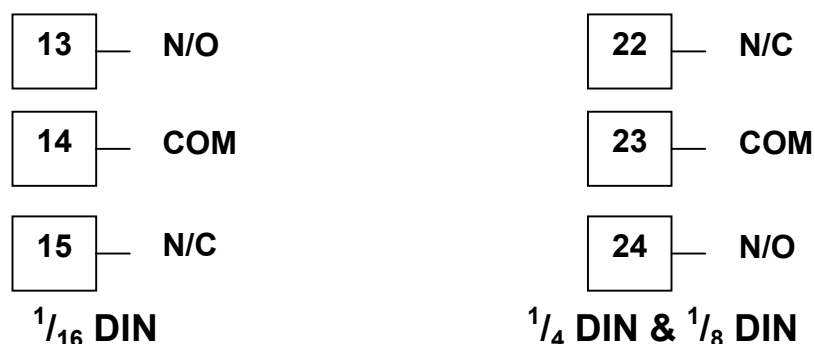
Figure 22. Option Slot 2 - Relay Module
