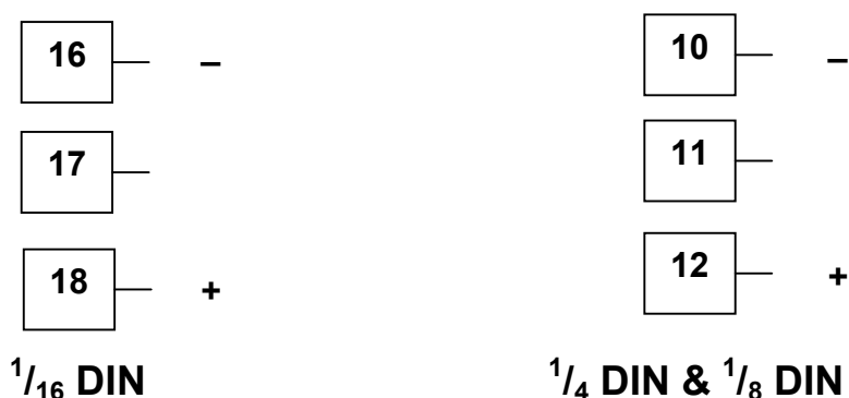
Figure 28. Option Slot 3 - SSR Driver Module
