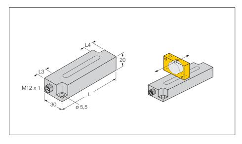
Blind zone connector end (L3) 5 mm Blind zone non-connector end (L4) 25 mm
