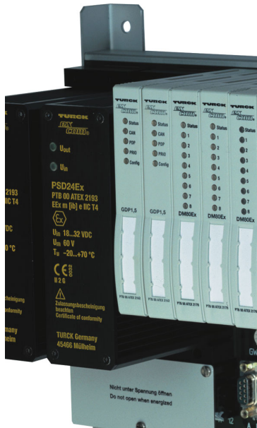
Figure 14: LEDs on gateways and modules
