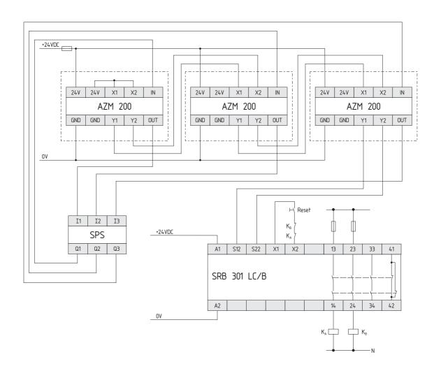
Wiring example: Series wiring of 3 AZM 200
