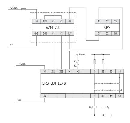
Wiring example: Single device wiring
