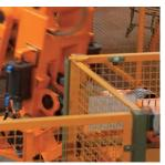
Solenoid interlocks demand accurate alignment of actuator and device. This requirement is met on new machinery. But during its lifetime, the situation may occur in which the actuator can no longer easily enter the device.
