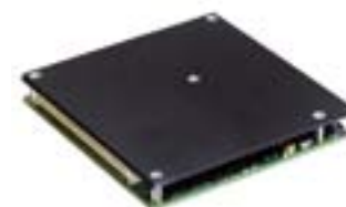
microETXexpress® with memory and heatspreader
