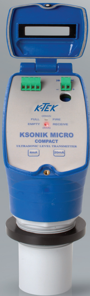
KSONIK™ KSONIK™ MICRO Compact Ultrasonic Level Transmitter and Switch ■ Up to 13 ft. / 4 m measuring range ■ Low cost, compact level transmitter with integral transducer ■ Temperature compensation ■ PVDF wetted parts for corrosive applications
