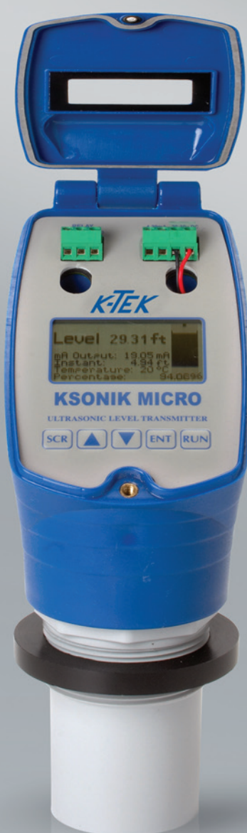
KSONIK™ KSONIK™ MICRO Ultrasonic Level Transmitter and Switch ■ Up to 32 ft. / 10 m measuring range ■ Low cost, compact level transmitter with integral transducer ■ 128 x 64 dot matrix display ■ Open channel flow measurement ■ PVDF wetted parts for corrosive applications ■ Continuous level transmitters and level switch ■ Trend recorder
