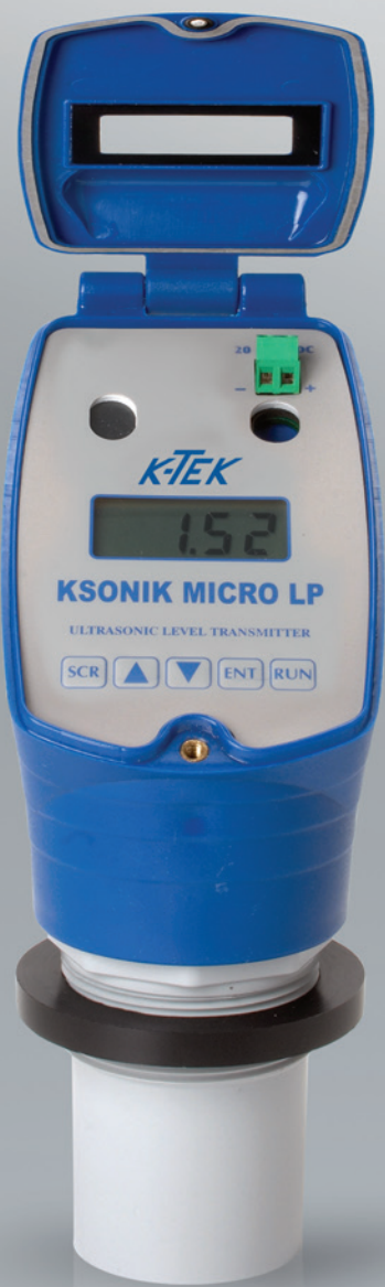
KSONIK™ KSONIK™ MICRO Loop Powered Ultrasonic Level Transmitter ■ Up to 16 ft. / 5 m measuring range ■ Low cost, compact level transmitter with integral transducer ■ Four digit alpha-numeric display ■ PVDF wetted parts for corrosive applications
