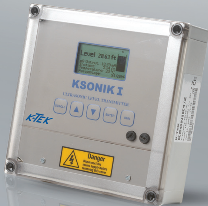
KSONIK™ KSONIK™ I Short Range Ultrasonic Level Transmitter ■ Range to 50 ft. / 15 m ■ Graphic LCD display ■ Integrated KSCOPE software ■ Automatic variable GAP for difficult applications ■ Open channel flow ■ Trend recorder
